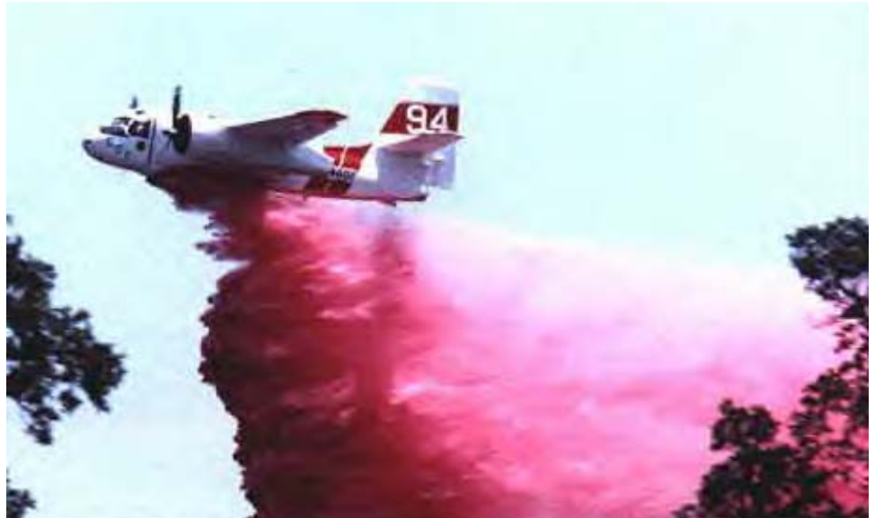
Figure 1 – Picture From Associated Air Tanker Pilot’s Web Site Showing A S-2 Air Tanker Dispersing Fire Retardant During Firefighting Operation
