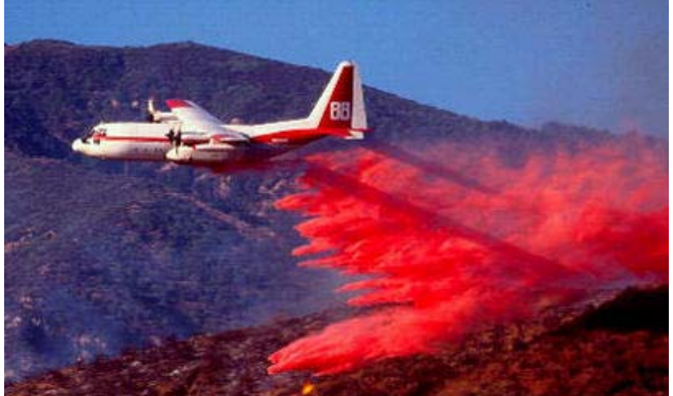
Figure 4 – Photo From Associated Air Tanker Pilot’s Web Site Showing A C-130A Air Tanker Dispensing Fire Retardant During Firefighting Operation
