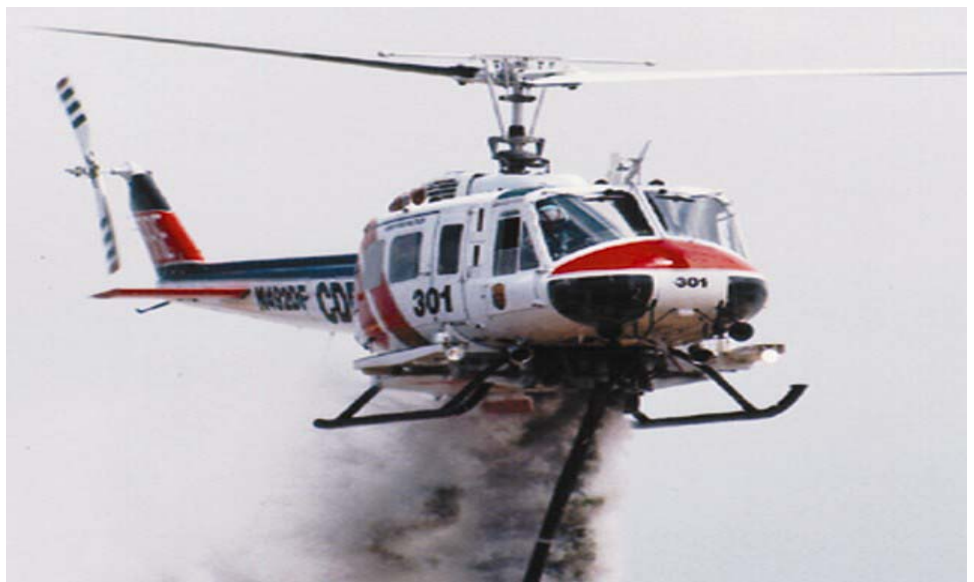
Figure 2 – California Department of Forestry Photo Showing A Tanked UH-1H Helicopter Dispersing Foam/Water During Firefighting Operation
