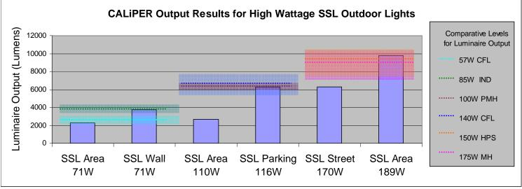
01/31/2008 Comparative levels are for initial luminaire efficacy and output, established using IES files and ballast factors for outdoor area lights, cobraheads, post-top, and pedestrian lights for CFL, induction, metal halide, pulse start metal halide, and high pressure sodium fixtures.
