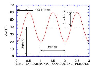
Figure 4: Sinusoidal component used in optional computation of boundary values from equations.
