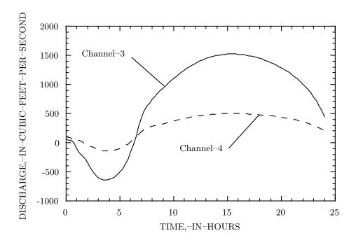
Figure 28: Flow in a simple six-channel network.
