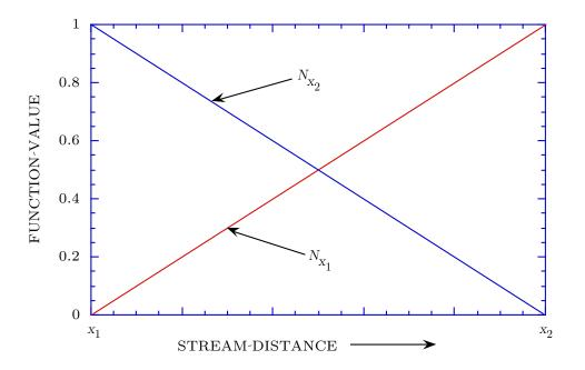
Figure 2: Linear interpolation functions.
