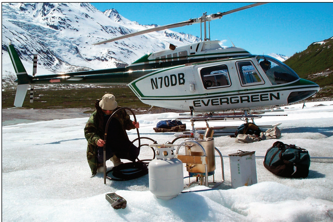
Figure 4. Propane-fired portable stream drill used to install ablation stake for measuring glacier melt on Tanaina Glacier (photograph by Rod March).
