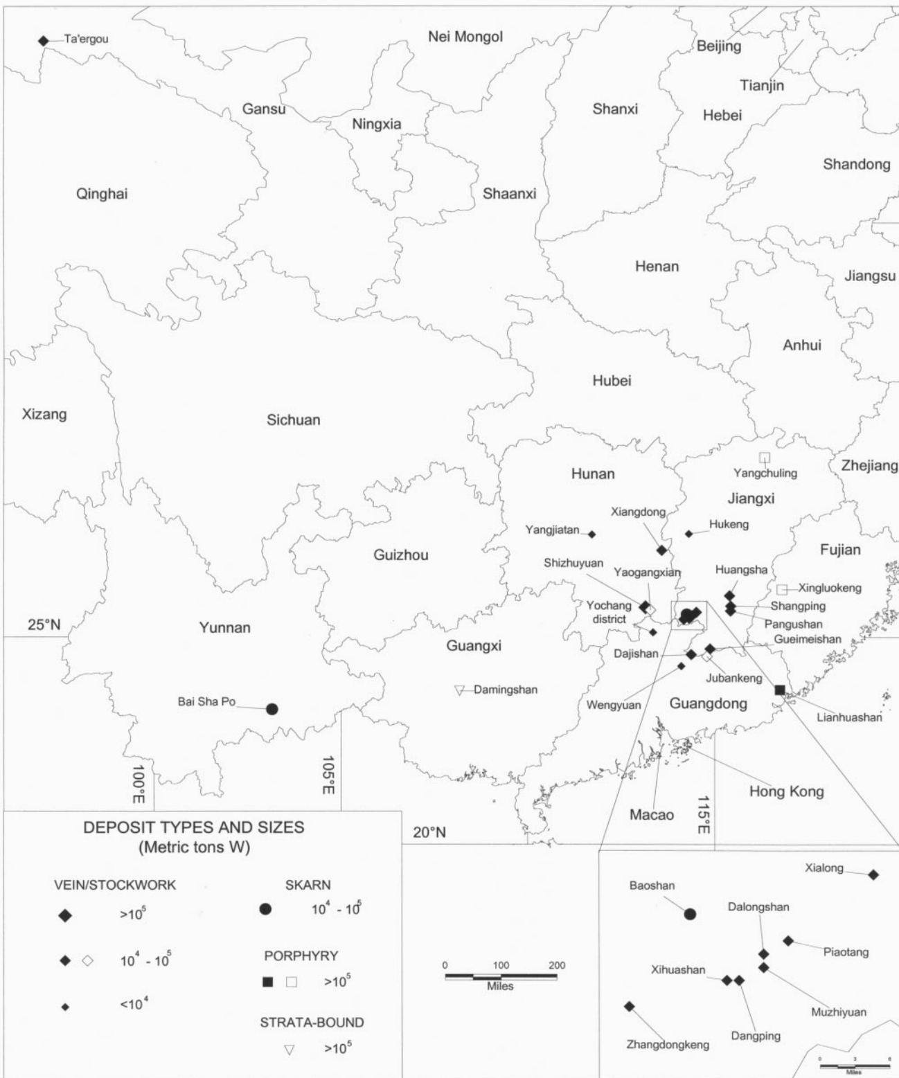
Figure 4. Location, type, and estimated resources of major tungsten deposits and districts in China. Resource data are from tables 9 and 10. Boundaries are not necessarily authoritative. Solid symbols indicate deposits in production in 1986; unfilled symbols indicate deposits not in production in 1986.
