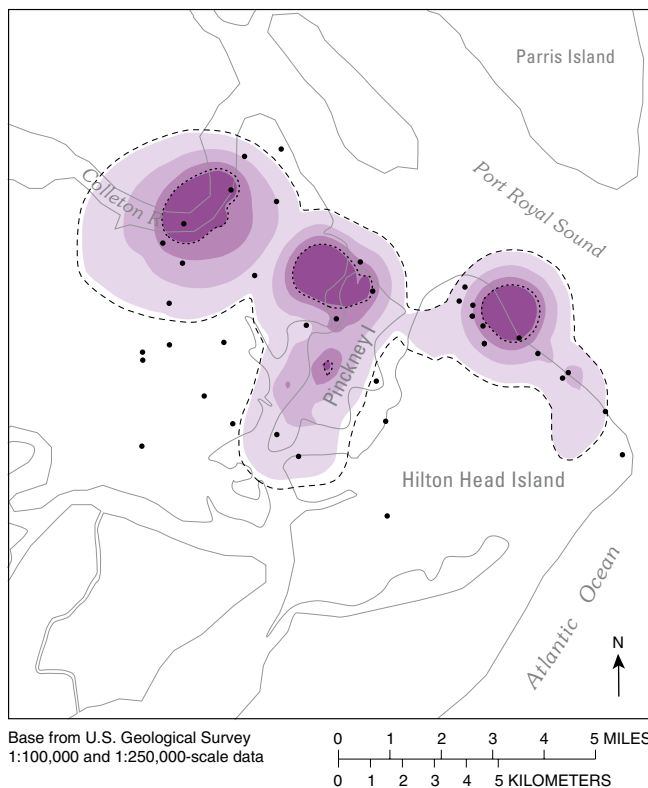
Figure 20. Simulated chloride concentration in ground water in the middle of the Upper Floridan aquifer in the Hilton Head Island, South Carolina, area for Scenario A (1997) (modified from Provost and others, 2006).
