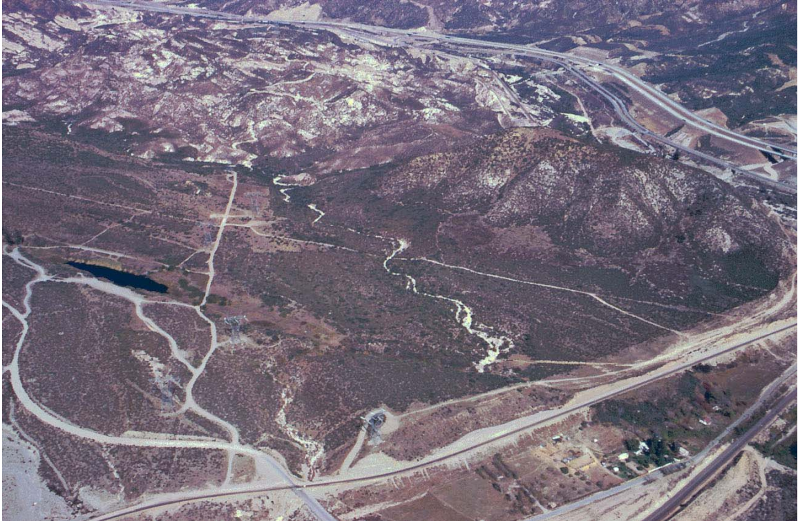
Photo 115. View north across lower Lone Pine Canyon. Lost Lake, a sag pond along the active trace of the San Andreas Fault is at the left center, and is elongate parallel to the fault. In the right center is the south end of a stream channel that is right laterally offset from the vicinity of the powerline tower to the right of Lost Lake. Light colored Cajon Valley Formation (Tcv) occupies the upper left part of the photograph. Interstate 15 is the highway in the upper part of the photograph.
