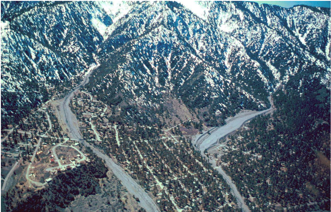
Photo 64. View looking south at the community of Wrightwood in Swarthout Valley (fig. 1). Wrightwood is built on debris-flow alluvial fans. The bare areas are the man-modified active debris flow channels of Sheep Creek (left) and Heath Creek. The dog-leg in Heath Creek channel results from an attempt to divert debris flows away from what was the extent of buildings in mid-20 th Century. Since 1969, debris flows have been deposited in the broad area of Heath Creek channel above the dog-leg. Major landslides originated at the heads of Sheep and Heath Creek Canyons (top edge of photograph).
