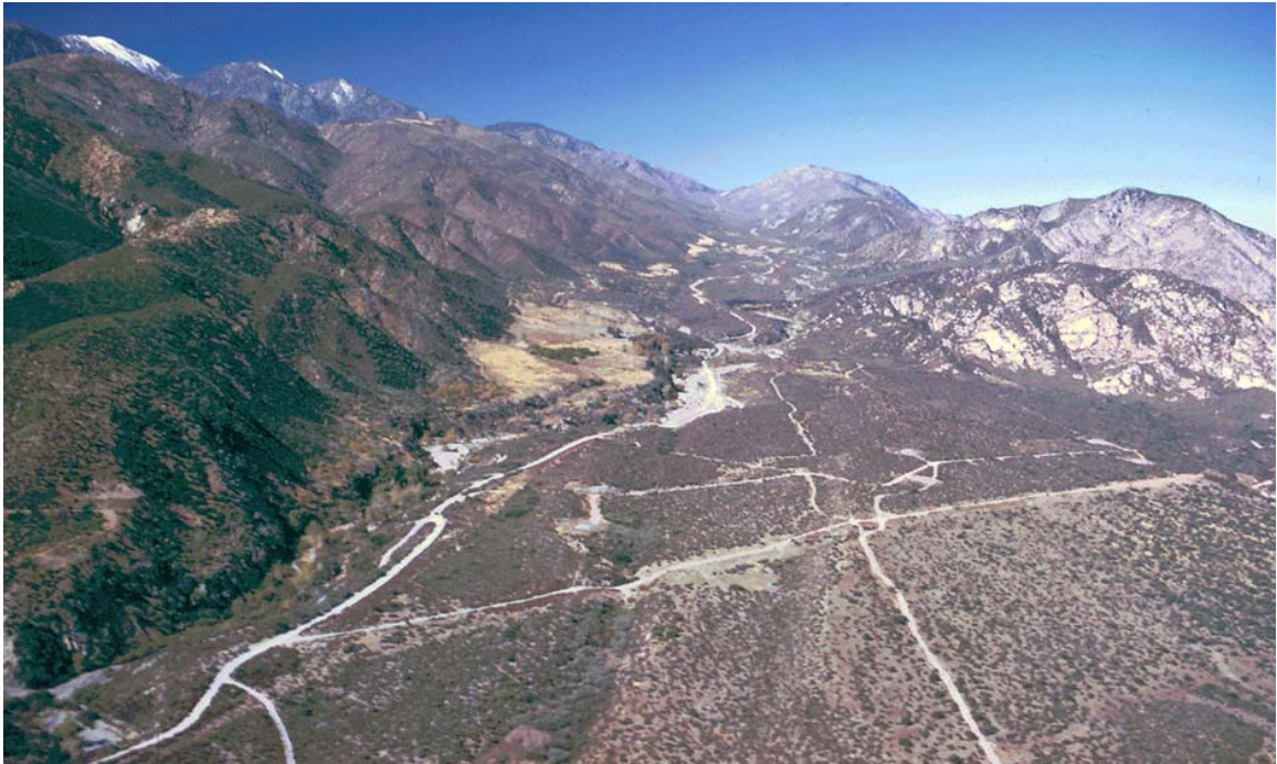
Photo 114. View west up Lone Pine Canyon, which is developed along the San Andreas Fault Zone. The most recent displacements are marked by the subtle scarp covered by brush, extending from lower center of the photograph to the notch in the skyline. Pelona Schist ( MzP ) underlies the ridge to the left of the valley and Cajon Valley Formation ( Tcv ) and older basement rocks ( MzPd ) are to the right.
