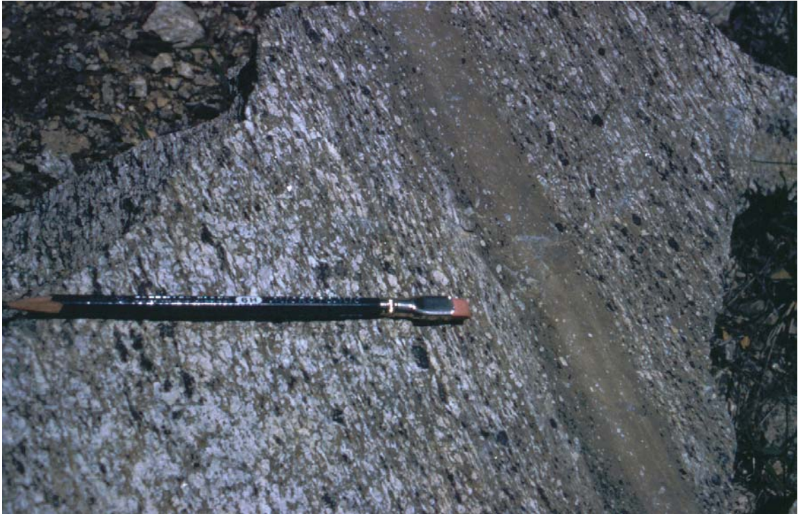
Photo 40. Well foliated cataclastic biotite-hornblende tonalite (Kssm 1 ) cut by seams of fine-grained mylonite. Note tectonically shaped plagioclase grains having tapered mineral trains at both ends. Photograph taken in San Sevaine Canyon area.
