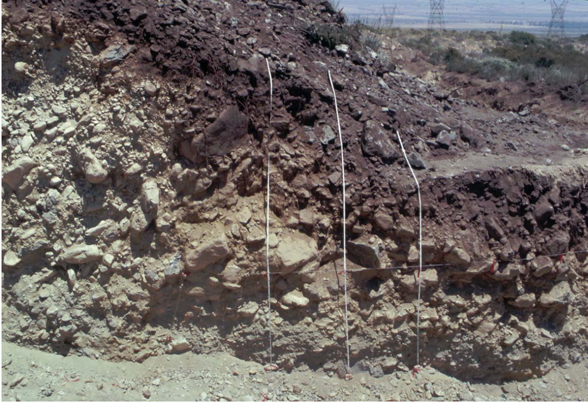
Photo 149. View to the east at the wall of a trench across the C scarp of the Cucamonga Fault Zone. The fault is marked by crude clast inbrication over a width of about 2 m about midway up the scarp (left side of the photograph). Dark colored fanglomerate to the left of the left vertical tape is where fan is being tectonically overridden.
