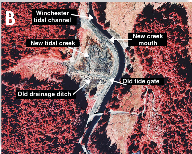
5.4. Creation of a new meandering tidal creek within the Dalton marsh, South Slough NERR, OR. A) Detonation of sub-surface explosives along the course of the new tidal creek bed (1998). B) Elimination of the old linear drainage ditch and re-establishment of hydrologic connection with the Winchester tidal channel through the new tidal creek (color IR air photo, 1999).
