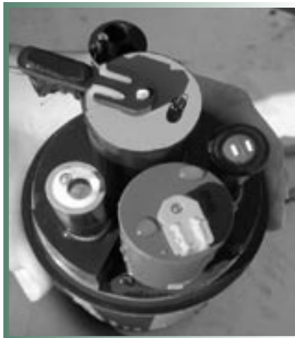
Multi-parameter sensor array on water quality datalogger
