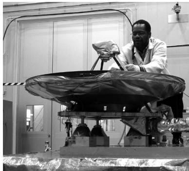
LEFT: An APL technician secures the electrical harness routed to the high-gain antenna on the STEREO "A" observatory. Credit: Johns Hopkins University / Applied Physics Laboratory
