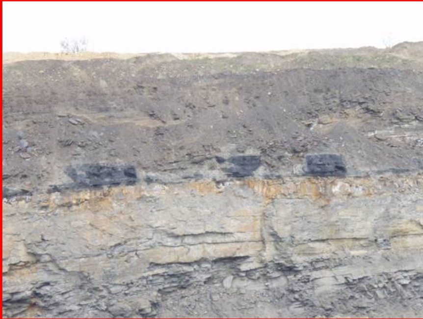
Figure 8. Pillars visible in the Sewickley seam retain square pillar corners despite total failure of the immediate roof and complete in-filling of old rooms. Layers of the immediate roof typify sag into the underlying rooms.
