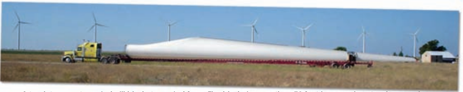
A truck transports a windmill blade to a wind farm. The blade is more than 70 feet long — almost as long as six cars.
