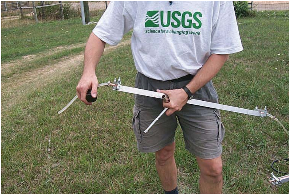
Figure 7. Collection of tritium/helium-3 age-dating samples.
