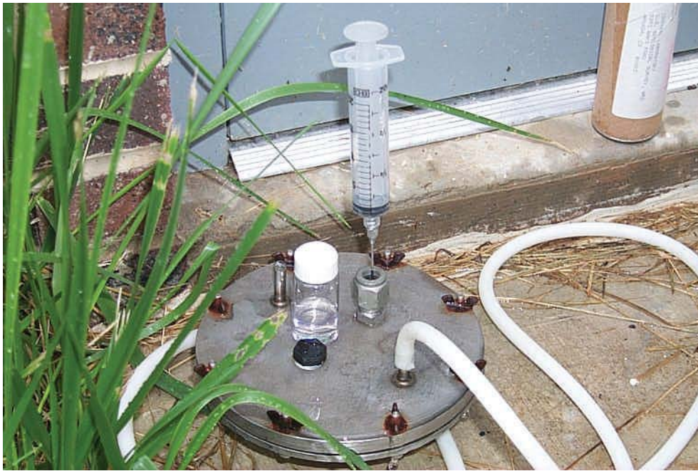
Figure 4. Flow chamber used to collect radon-222 sample.
