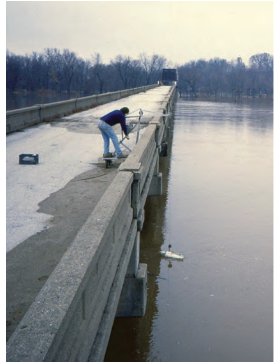
Large streams and rivers required sampling from bridges, boats, or cableways.
