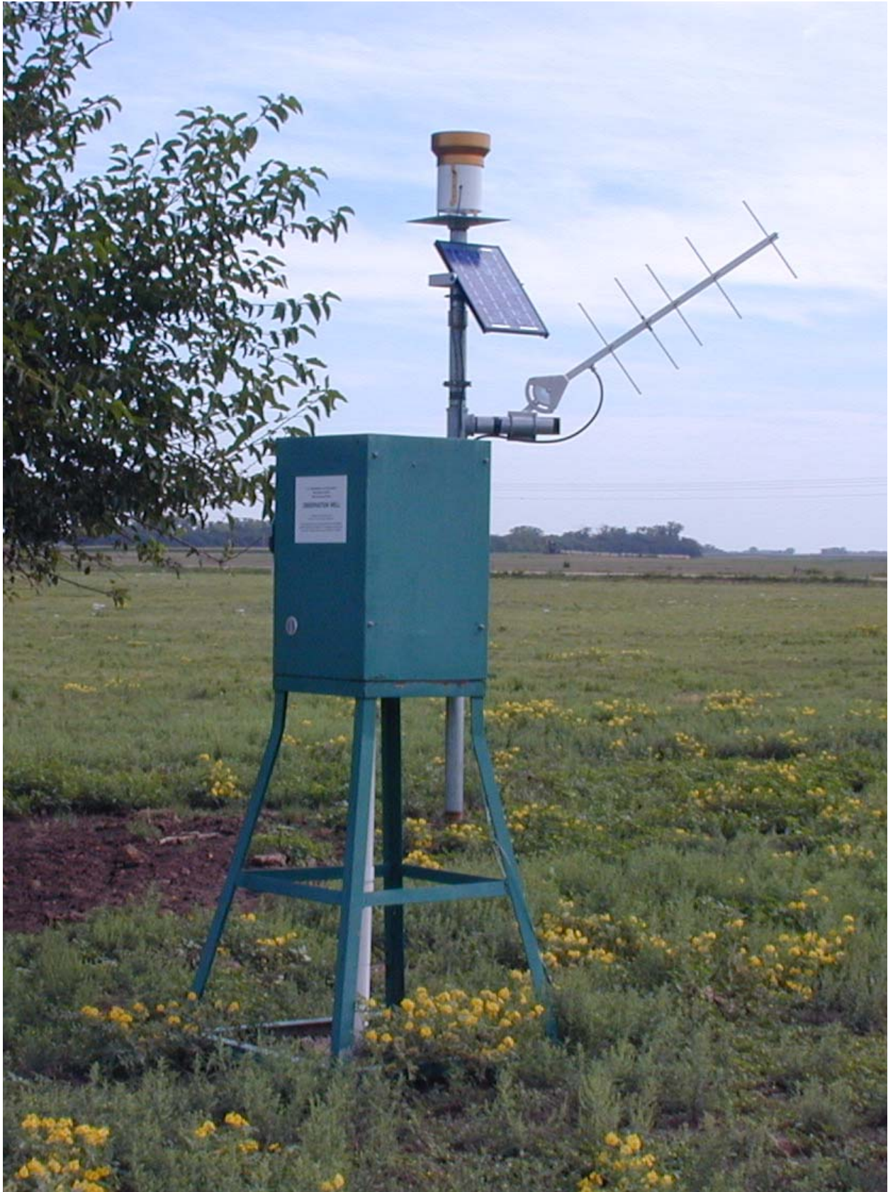
Real-time ground-water-level monitor at Stafford County well at 21S-13W-27DDDC01. Photograph courtesy of R.W. Gauger.
