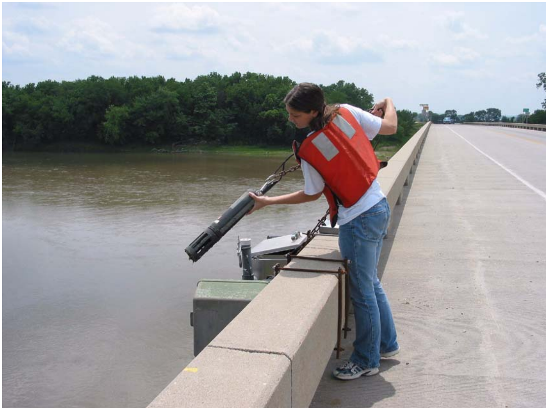
Deploying water-quality sensor at Kansas River near DeSoto (station 06892350, fig. 1). Photograph courtesy of L.C. Millikan.
