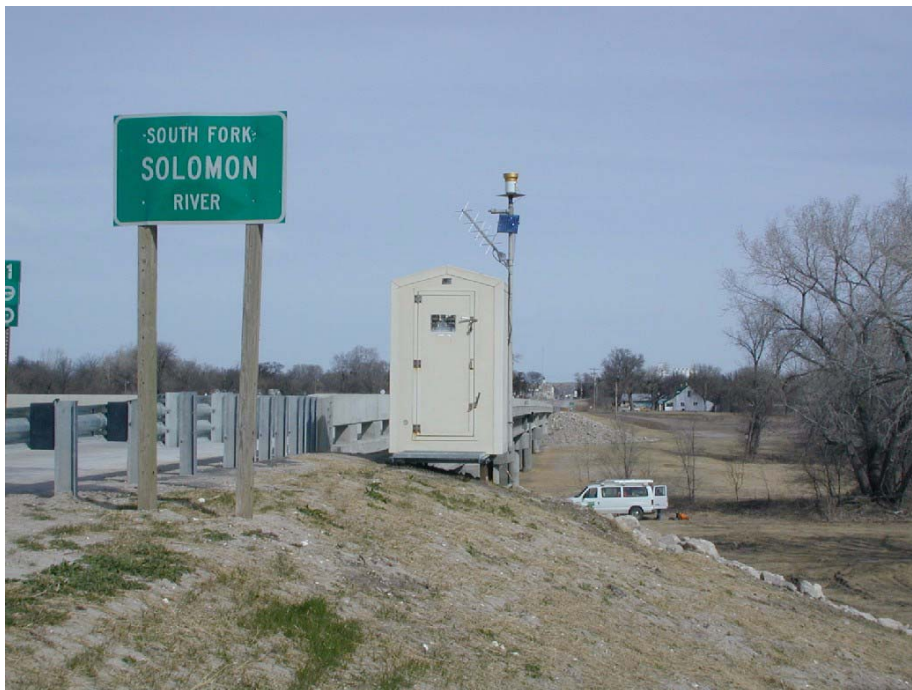
Streamflow-gaging station on South Fork Solomon River at Osborne. Photograph courtesy of C.A. Dare.
