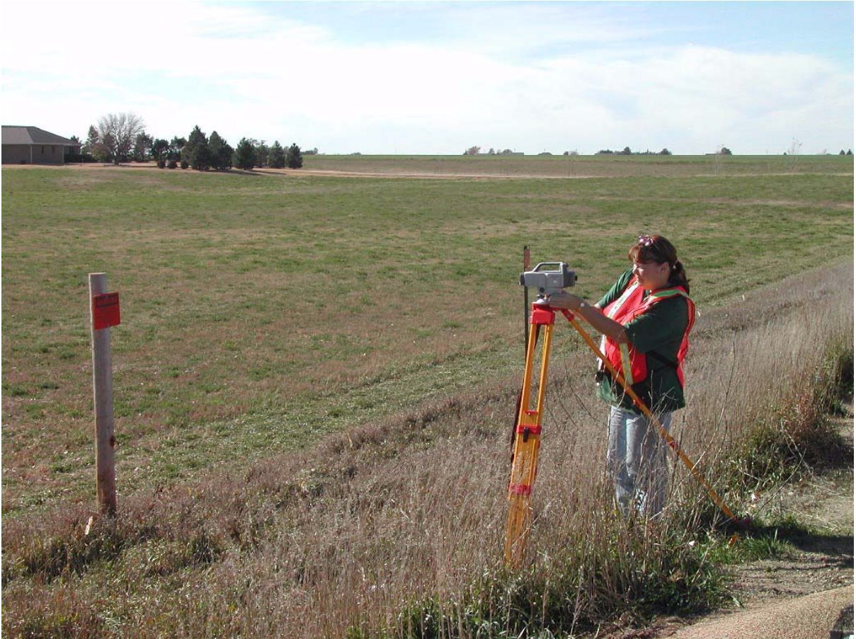
USGS technician prepares for survey of reference point elevations at partial-record station. Photograph courtesy of L.S. Hill.
