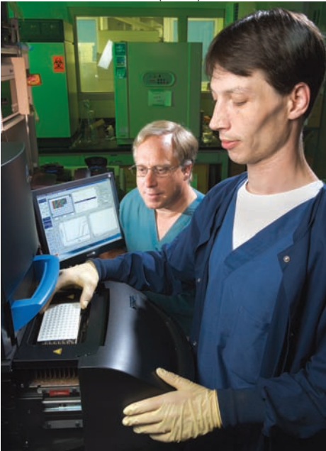
Microbiologist John Neill (left) and technician Bill Boatwright load samples into a fluorescent real-time thermocycler to measure levels of mRNAs present in BVDV-infected cells. This data is used to confirm results obtained from SAGE analysis of the same cell population.
