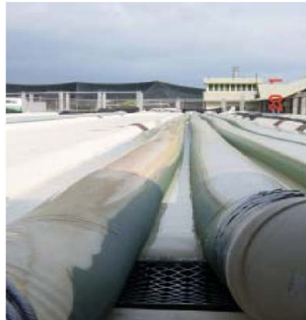
The Aquasearch Growth Module is a commercial-scale closed photobioreactor
