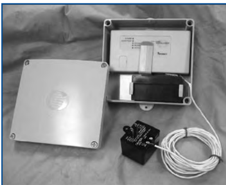
Figure 4. Repeater in NEMA Box with backup battery and power adapter.
