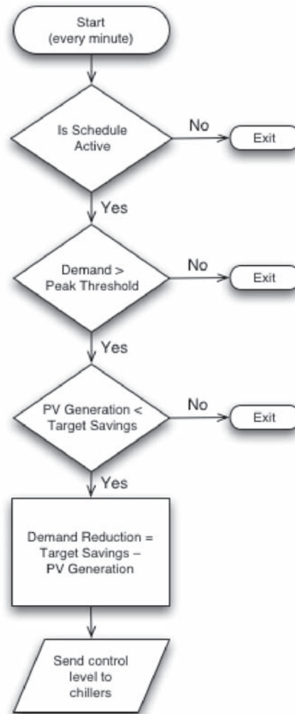
Figure 8. SLC control logic.
