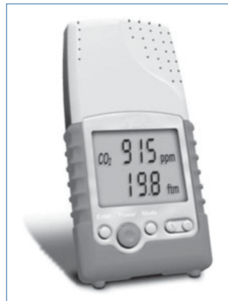
Figure 2. Typical non-dispersive infrared spectroscopic CO 2 sensor.
