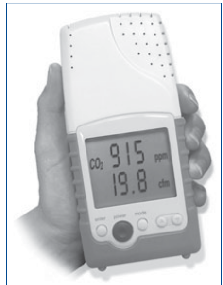
Figure 5. Handheld CO 2 sensor with cfm/person calculation and data logging.
