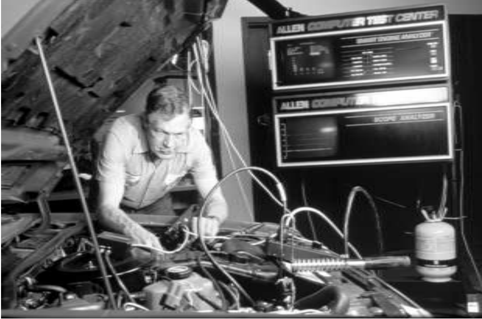
A technician performs a quality inspection of an aftermarket-conversion AFV that runs on ethanol.
