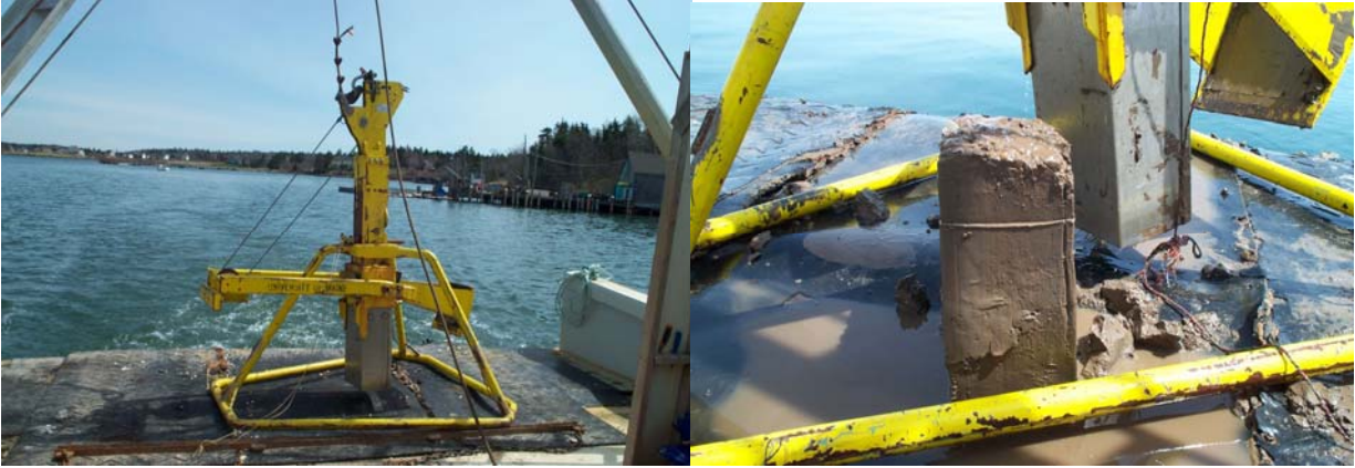
Appendix A8. Figure 9. Ocean Instruments 610 Boxcore along with a typical core sampled.
