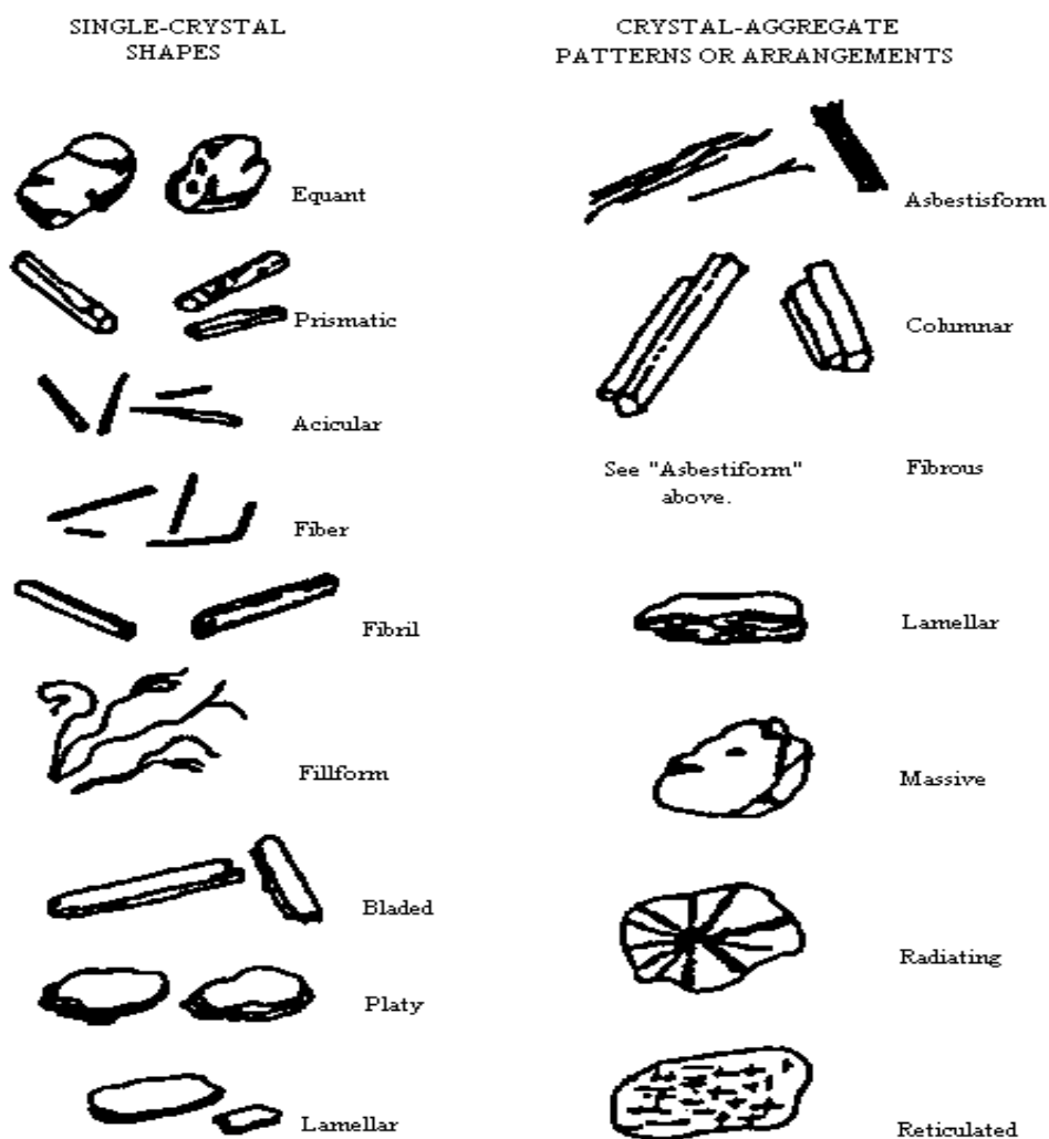
Figure 1. Particle definitions showing mineral growth habits. From the U.S. Bureau of Mines
