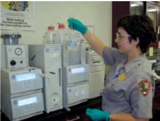
NPS hydrologist Katie Seadler, for the Cumberland-Piedmont Network (stationed at Mammoth Cave NP), analyzes water samples for anions, cations, trace metals and pesticides using an Ion Chromatograph.
