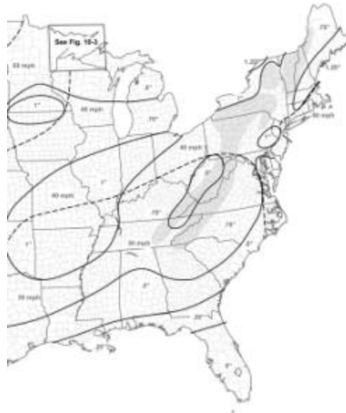
Figure 10-2. 50-year mean recurrence interval uniform ice thicknesses due to freezing rain with concurrent 3-second gust wind speeds: contiguous 48 states.
