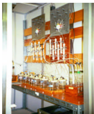
Figure 8. Flow-through Microcosm Test System.
