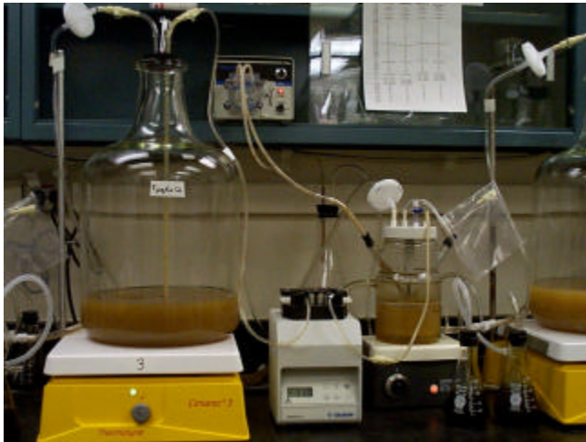
Figure 6B. A photograph of the chemostat in operation. The large vessel on the left is the feed vessel. The small spin-flask with multiple ports is the culture vessel, and contains 500 ml of a steady-state culture of colonic bacteria. The waste vessel is located behind the culture vessel and peristaltic pump.
