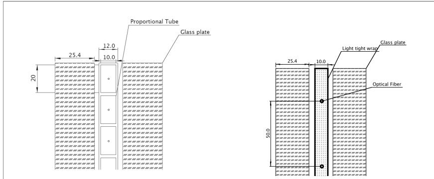
Proportional tubes ArCo2 (80:20) Gain of 3000 gives 52 fC 250 tubes per plane 500k-1000k total channels
