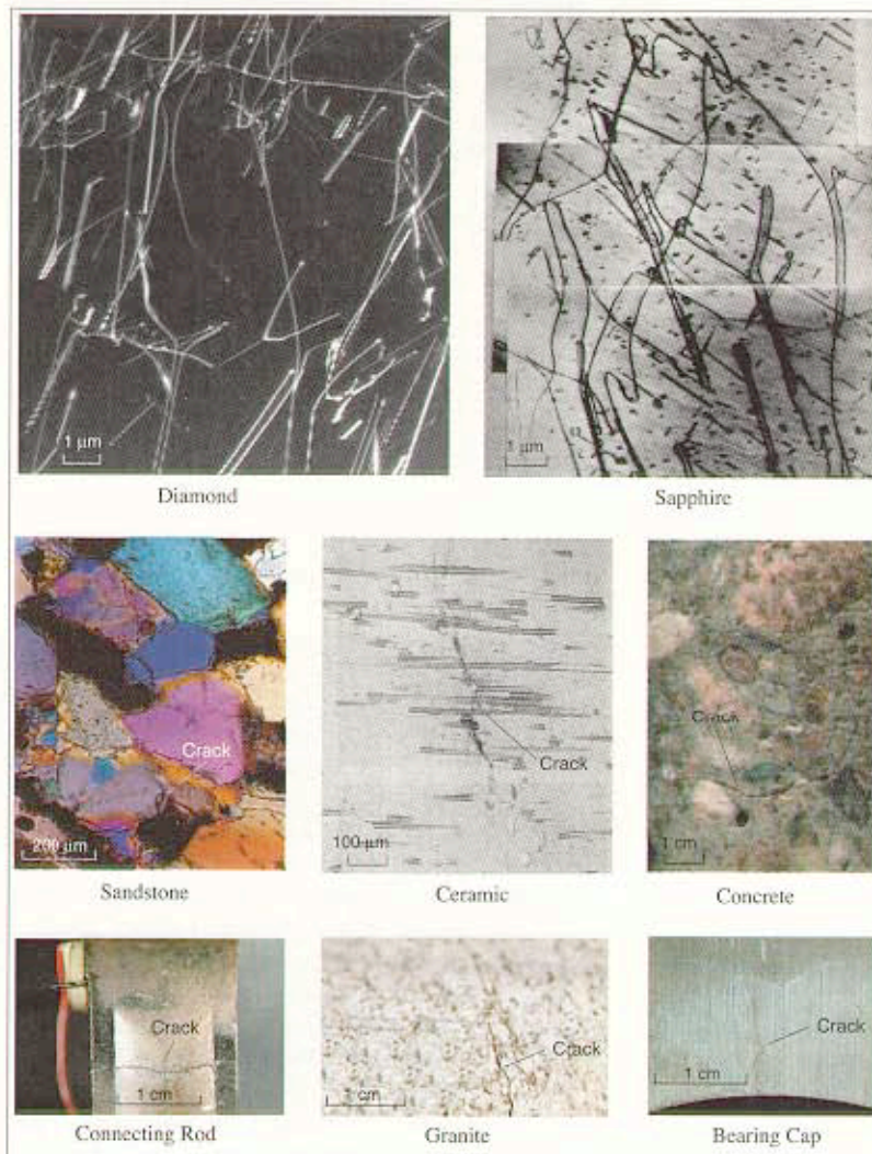
Figure 4 Photomicrographs and photographs showing features that can provide a nonlinear response to the bulk material when excited in a wave field
