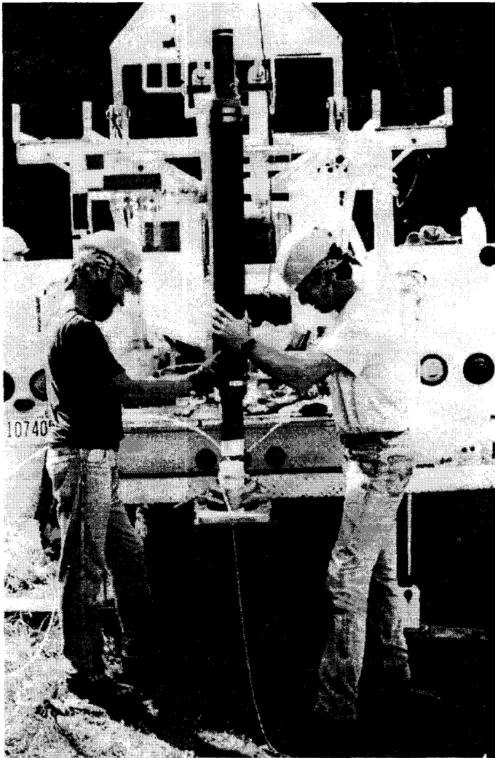
Figure 2. One of the log-through packers being installed. The inflatable rubber bladder is 1 m long and is installed over a plastic pipe to allow borehole tools to be operated through the packer. Metal was minimized, but two metal clamps, similar to automotive radiator hose clamps, are located near each end, and small metal eye-bolts are located at the top of the packer section. Tubing for compressed air is also visible. (Photograph courtesy of Peter Joesten, USGS)
