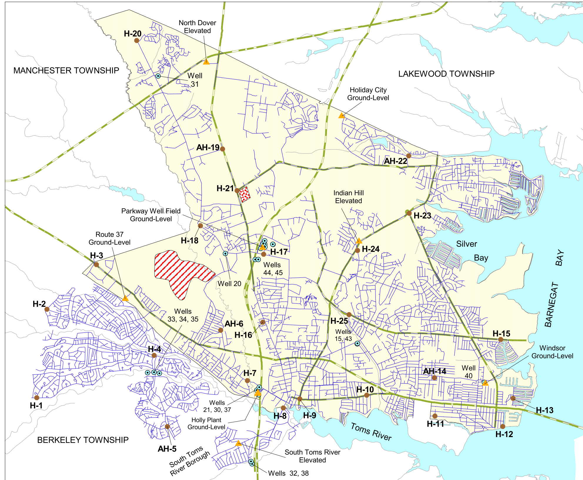
PLATE 6. LOCATIONS OF TEST HYDRANTS USED FOR INSTALLATION OF PRESSURE DATA LOGGERS TO COLLECT SYSTEM-WIDE PRESSURE DATA, DOVER TOWNSHIP AREA, NEW JERSEY
