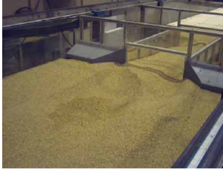
Figure 25. Photo. Outlet scour after test.
