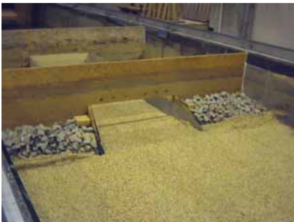
Figure 28. Photo. 8-degree inlet wingwalls before scour.
