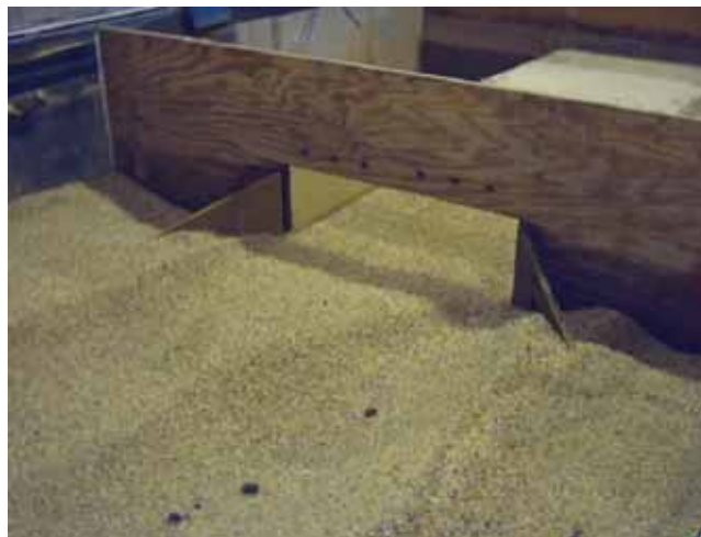
Figure 40. Photo. 45-degree wingwalls after scour.
