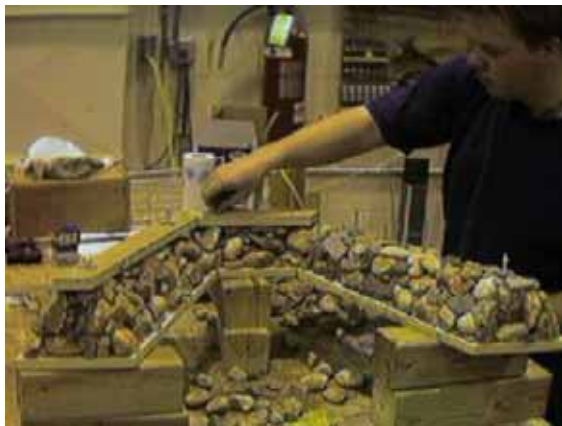
Figure 58. Photo. Fabrication of the cross vane.
