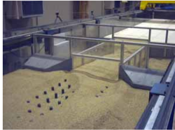
Figure 45. Photo. Outlet scour area with protective pile dissipators.
