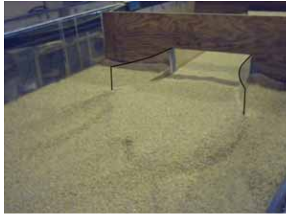
Figure 34. Photo. Elongated, streamlined wingwalls after scour.
