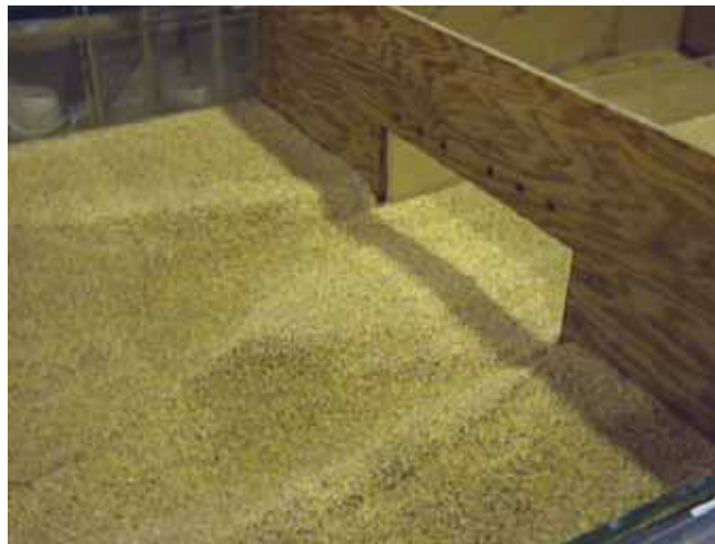
Figure 30. Photo. No wingwalls.
