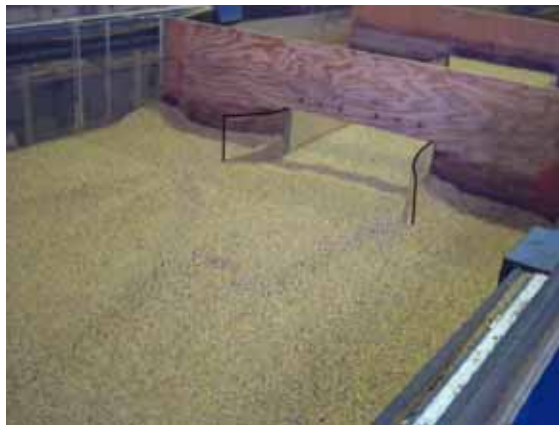
Figure 35. Photo. Short, streamlined bevel wingwalls after scour.
