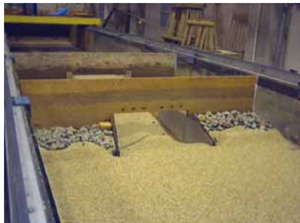
Figure 29. Photo. 8-degree inlet wingwalls after scour.
