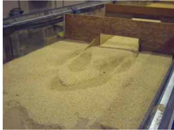
Figure 37. Photo. Wingwalls with 8-degree flare (rough joint) after scour.
