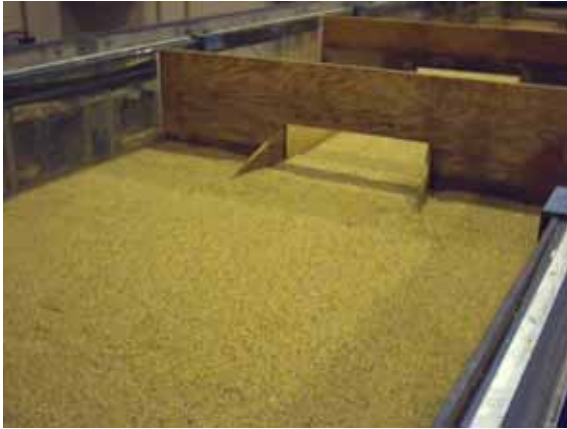
Figure 36. Photo. Wingwalls with 8-degree flare (rough joint) before scour.
