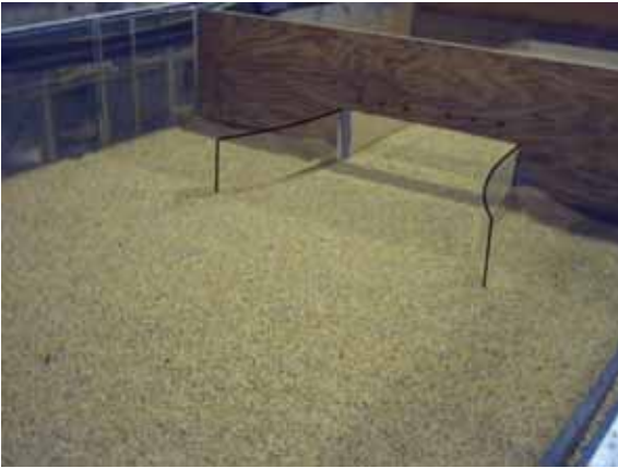
Figure 33. Photo. Elongated, streamlined wingwalls before scour.
