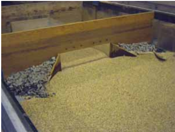
Figure 26. Photo. 45-degree inlet wingwalls before scour.
