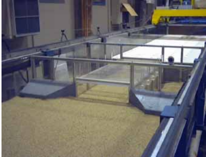
Figure 43. Photo. Culvert outlet prior to pile dissipator test.
