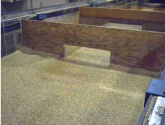
Figure 31. Photo. Truncated, circular wingwalls before scour.
