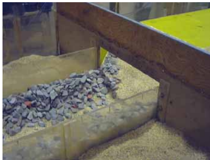
Figure 52. Photo. Shifted riprap in culvert barrel after Standard Plan test.
