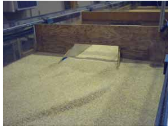
Figure 39. Photo. Wingwalls with 8-degree flare (smooth joint) after scour.
