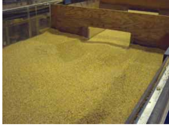
Figure 32. Photo. Truncated, circular wingwalls after scour.
