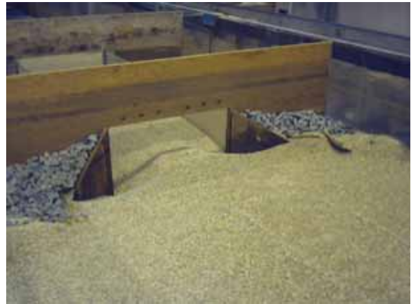
Figure 27. Photo. 45-degree inlet wingwalls after scour.
