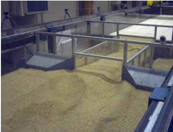
Figure 44. Photo. Outlet scour area without protective pile dissipators.
