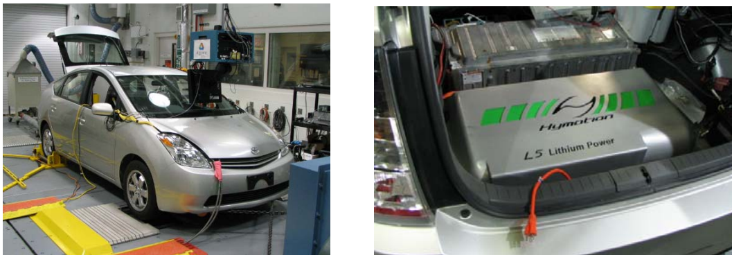
Figure 1: Hymotion PHEV Prius on Chassis Dynamometer with Hymotion 5-kWh Battery System Installed in Parallel to the Production Battery
