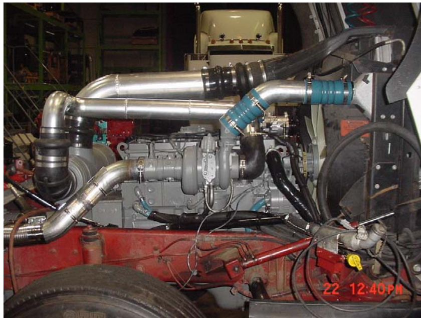
Figure 8: Alpha Engine Installation
