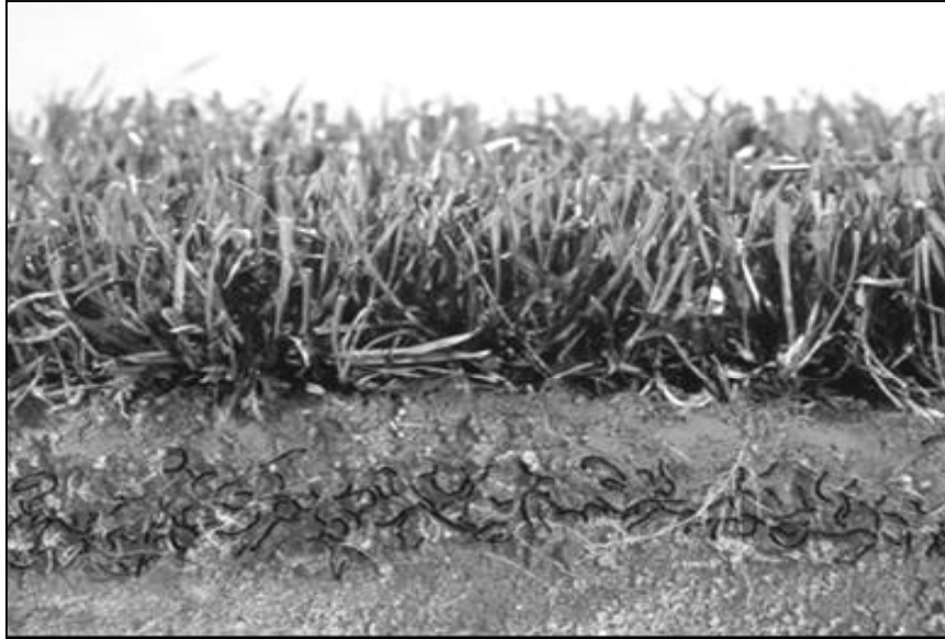
Figure 1.7. TRM Profile with Vegetation/Soil/TRM Matrix (Source: ECTC)
