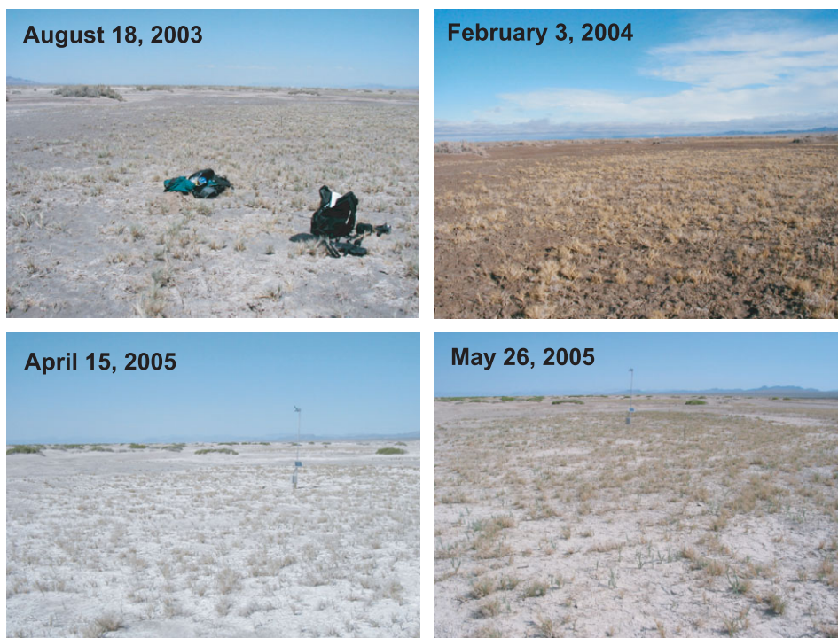
Figure 4. Repeat photographs at Discovery site, Franklin Lake playa. Surface in August 2003 consisted mainly of gray silt with remnants of white fluffy evaporate-rich sediment near clumps of saltgrass. Efflorescent salts were removed by heavy rainfall on February 2 2004 as shown in the photograph taken the next day. On April 15 2005 the surface consisted of extensive fluffy efflorescent salts that were subsequently removed by wind erosion, as shown in the photograph taken on May 26 2005.
