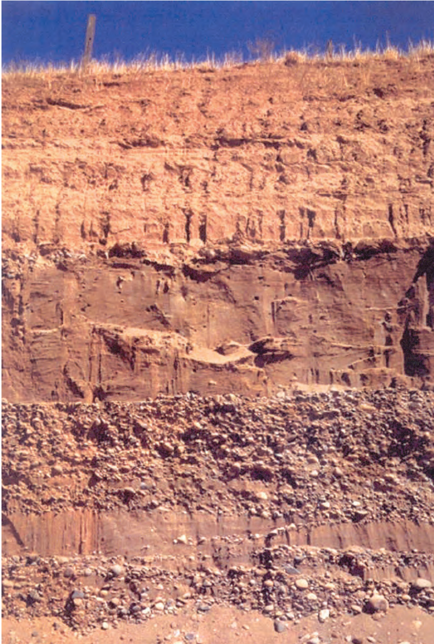
Figure 3. An alluvial deposit near Sacramento, California, that exhibits heterogeneity and vertical anisotropy where a 1- to 2-meter-thick, silty-clay layer at the ground surface is underlain by sand, sandy gravel, and gravelly sand layers. (Photograph from Boulanger and Duncan, 2000)
