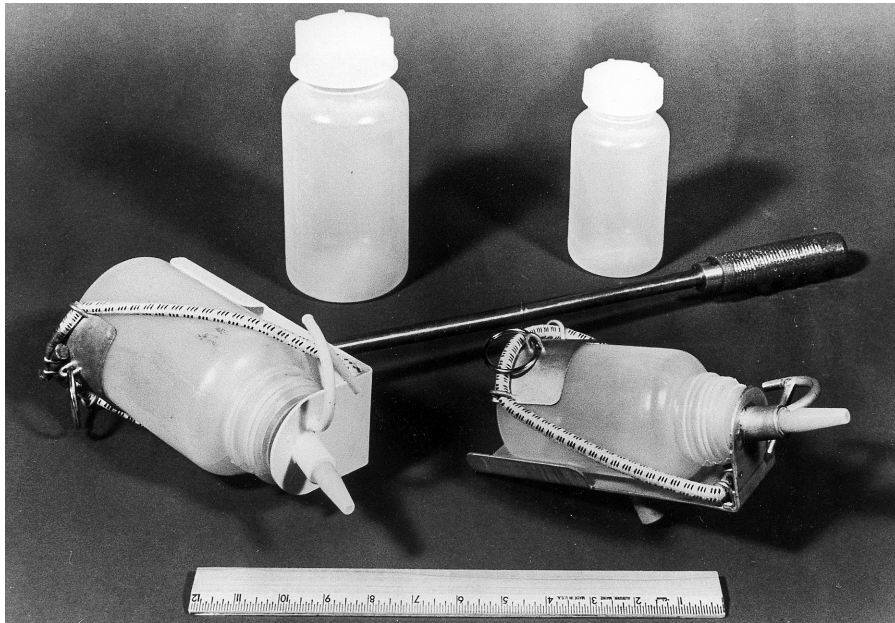
Figure 3. US DH-75 (P and Q) suspended-sediment samplers with sample containers and wading rod.
