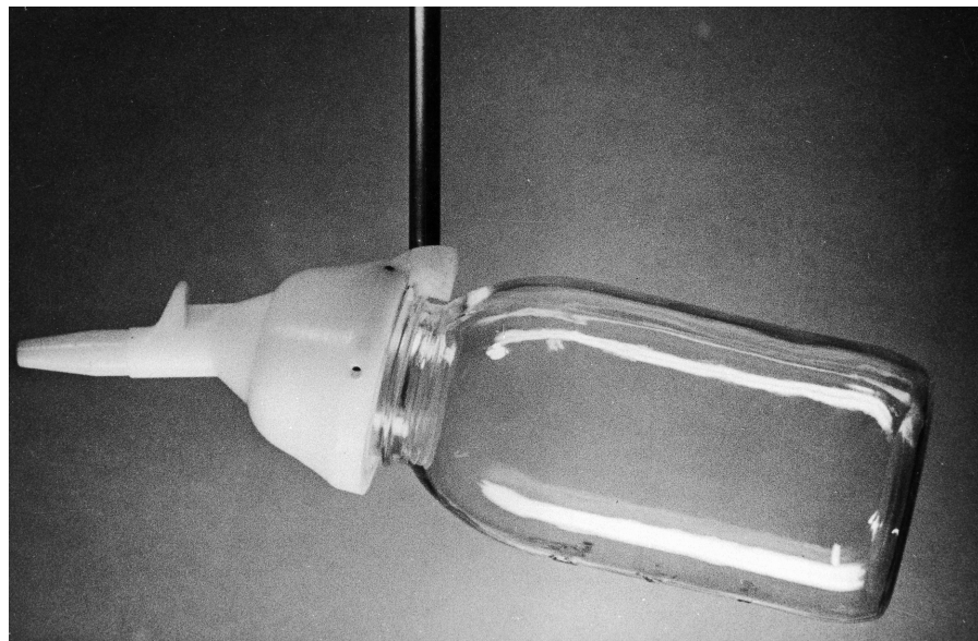
Figure 2. US DH-81 suspended-sediment sampler shown with a US DH-81A adapter, D-77 cap and nozzle, wading rod handle, and quart glass bottle.
