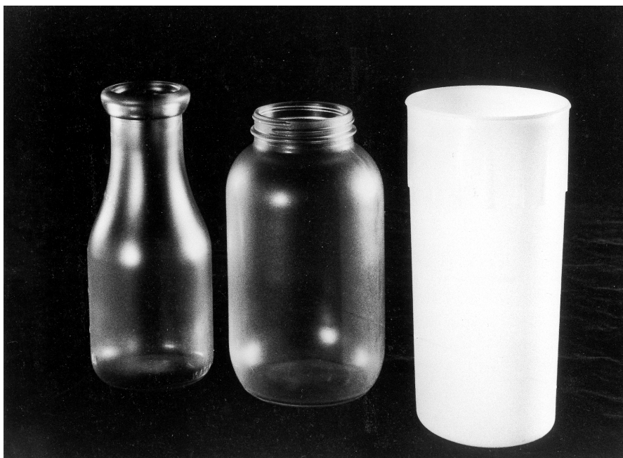
Figure 12. Sample containers to fit PS-69 pumping sampler (left to right): pint glass milk bottle, quart glass mayonnaise bottle, and quart plastic container to fit the PS-69 pumping sampler.
