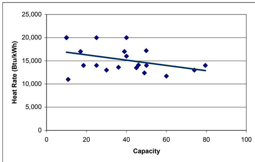
**Figure 12-2. Reported heat rate for 20 operating biomass plants<sup>112</sup>**
