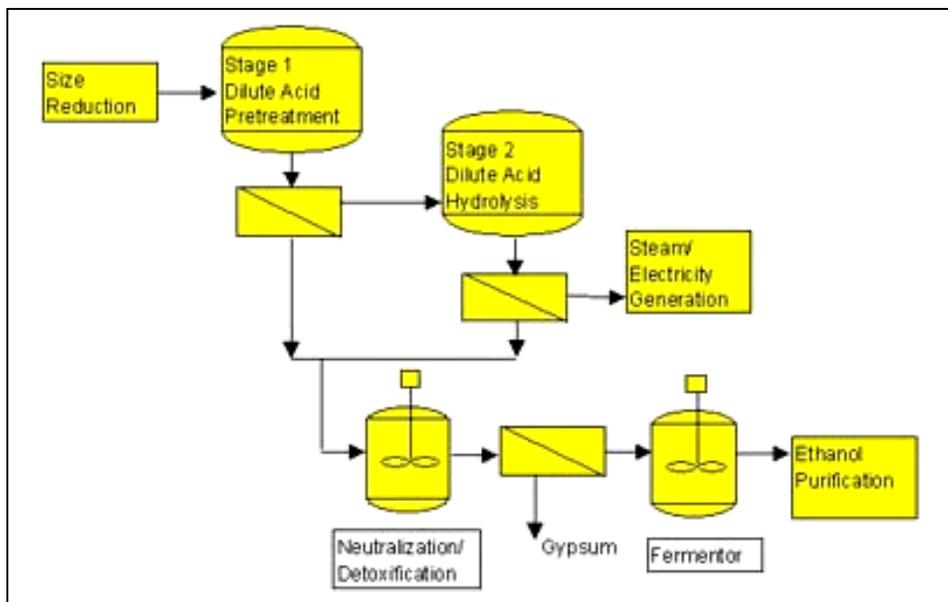
**Figure 12-9. Example process flow for dilute acid hydrolysis**
