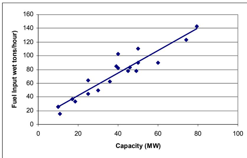
**Figure 12-4. Biomass fuel consumption based on 20 operating facilities<sup>113</sup>**
