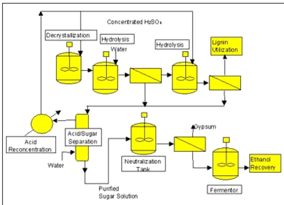
**Figure 12-8. Example process flow for concentrated acid hydrolysis**
