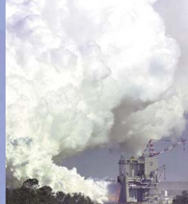
1969: Test-firing an S-II booster
