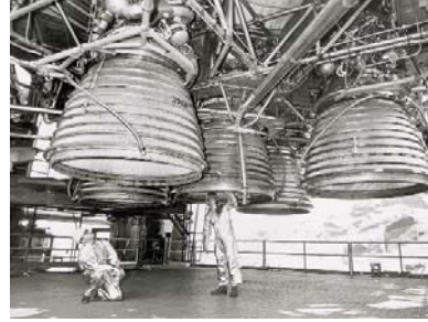
1966: Workers prepare J-2 engines for testing
