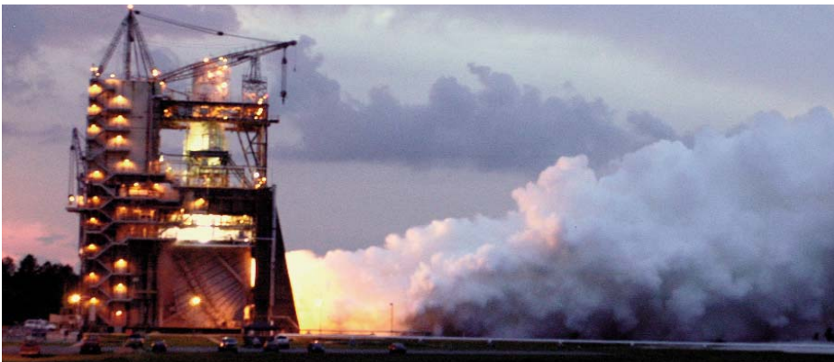
2004: Test of a space shuttle main engine for NASA's Return to Flight after loss of space shuttle Columbia
