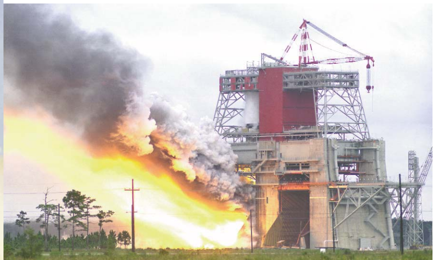
1967: First test-firing of a Saturn V booster stage, a cluster of five F-1 rocket engines
