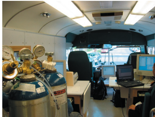
Interior of the EPA's trace atmospheric gas analyzer (TAGA) bus. TAGA was used for real-time sampling of residences near the Chillum site.
