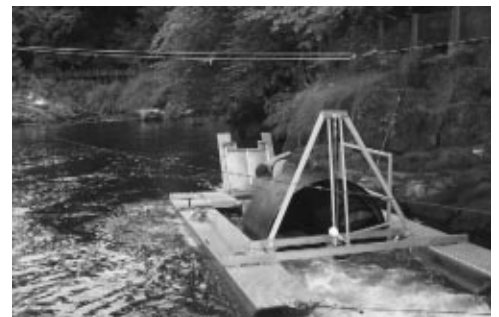
It’s a... screw trap. Downstream migrating juvenile Pacific lamprey enter the trap through the cone, which has a cork-screw fin in it that turns the cone when water hits it. As the cone spins, all fish are funneled into the live box, where they remain until the trap is checked. At the back of the live box is a perforated debris drum that removes floating debris from the box. FWS photo: Scott Barndt.
