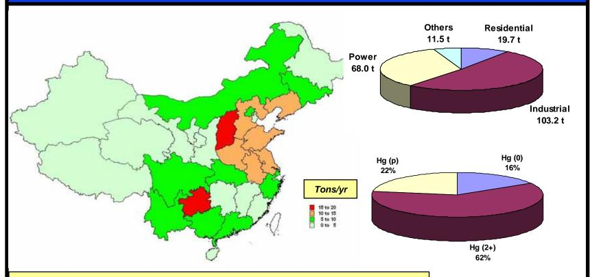
Total Hg emissions from coal combustion: 202.4 tons
