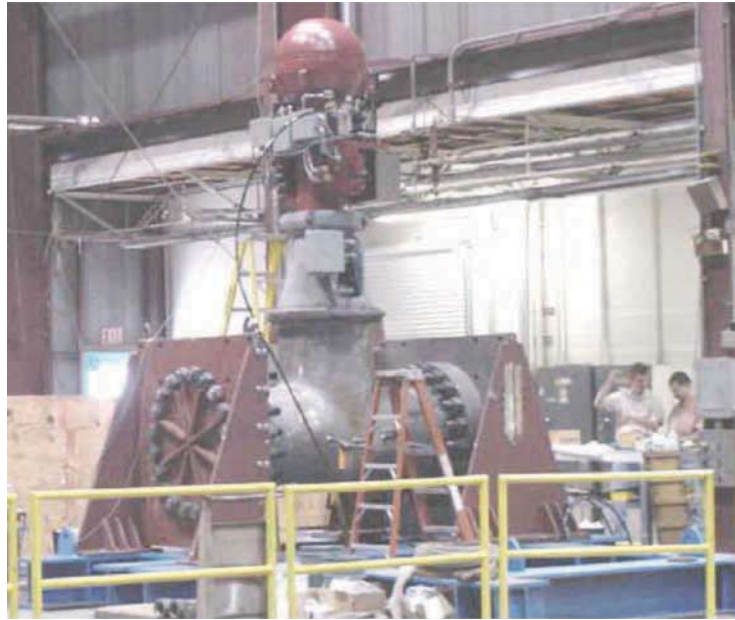
Figure 3 Size 26 x 24 x 26 Main Steam Isolation Valve
