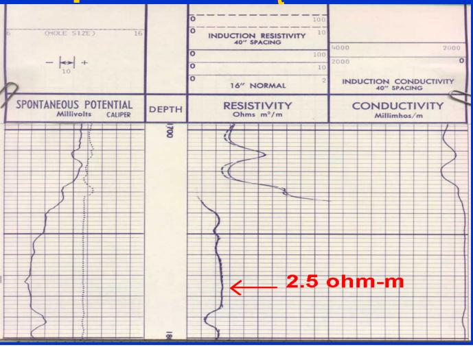
• This analysis requires a resistivity, induction, or Laterlog-type well log, although you can even use a value from a pre-1940 "electric log." Choose a log value for formation resistivity in a clean, permeable, thick (>5 feet) bed. If you are using a resistivity log, use a "deep-focused" curve. Always watch the scale, and make sure you have the decimal in the right place. In this case, the value is 2.5 ohm-meters.
