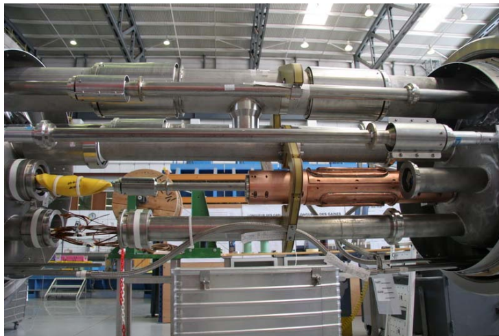
Q2-Q3 interconnect, including TAS B absorber around beam tube
