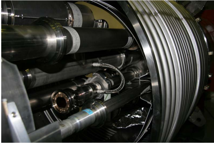
Q1-Q2 interconnect, including plug-in module
