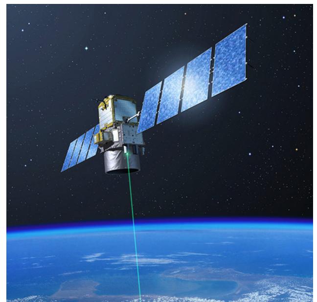
Figure 1: An artist's rendition of what the CALIPSO satellite would look like from space. Using pulses of laser light from an instrument called a lidar, CALIPSO takes global measurements of the atmosphere, studying small particles in the air, called aerosols, and multi-layered clouds to better understand Earth's weather, climate and air quality. (Image courtesy of CNES.)
