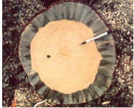
Figure 4 —Sapwood has been discolored by blue-staining fungi; heartwood is not stained.
