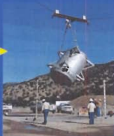
40 inch drop onto 6 inch steel spike
