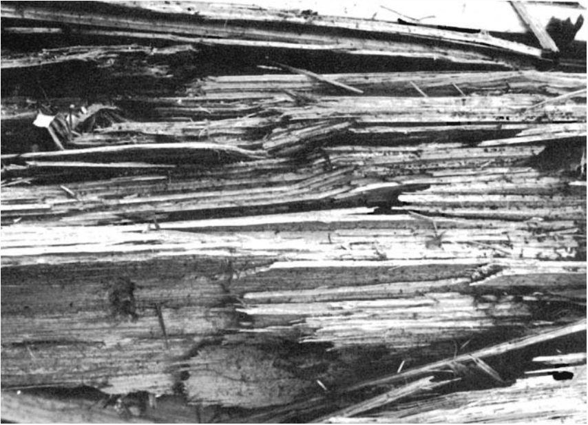
Figure 6. —Longitudinal section of a broken grand fir log containing a late stage of rust-red stringy rot, showing separation of the wood along the annual rings.
