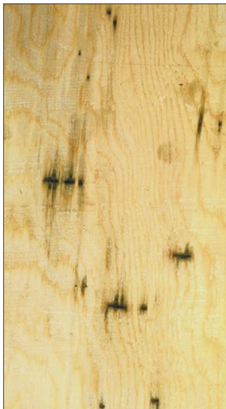
Fig. 5. Plywood veneer showing pinholes and stain from ambrosia beetle infestation.
