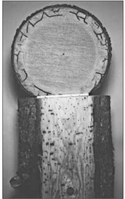
Fig. 3. Sections of Douglas-fir log showing T. lineatum galleries and pinhole appearance.
